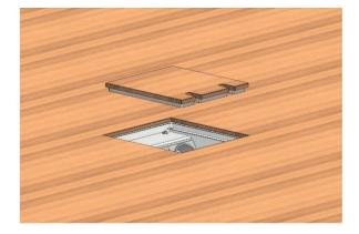
Cut the lid from floor material (Be careful about wood patterns!), size 240x240mm or depends on size of the hole made for the box. Glue aluminium lid (235x235mm) to the lid from floor material; be sure it's glued in the centre. Cut openings in relevant places for electric cords. If multiple holes not needed, you don't have to cut them out)
