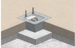
Rest of the empty space around floor box is filled by glue/mortar etc. Fill it to the same level as surrounding concrete floor. Prepared wires will connect to corresponding sockets and socket holder is inserted back.
